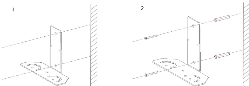
Use the bracket to mark and drill the necessary holes in the wall. \*NOTE: wall anchors are for illustration only, and are not included.
