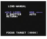
ELC Levels and DC Levels are adjustable. The higher the number, the brighter the image.
