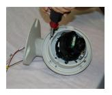
3 Attach the camera to the wall mount housing.
