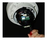
Attach the camera to the junction box using the machine screws.
