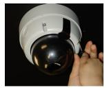
Attach the camera housing to the junction box using the assembly screws.
