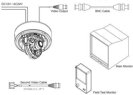
Power Connection: 12VDC & 24VDC Dual Voltage (Auto Polarity Detection and Protection) All cameras are equipped with a second video output for on-site configuration.
