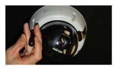
Attach the camera housing to the junction box using the assembly screws.
