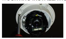
• Pull wires through and make connections. Refer to page 13. Use mounting template to mount camera with drywall mounts and machine screws.
