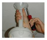
Use the mounting template to make pilot holes. Mount the camera assembly to the ceiling using wall mount anchors and machine screws.
