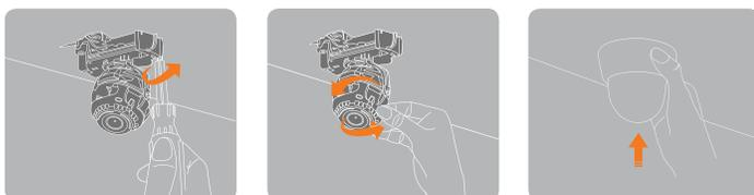
1 Two Screw Installation      2 Adjustment      3 Snap It
